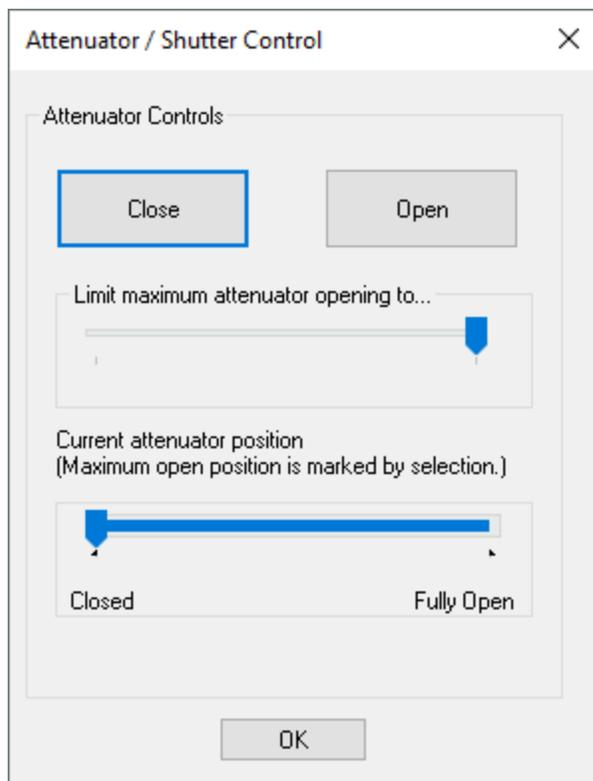
Figure 57: The Attenuator / Shutter Control dialog
