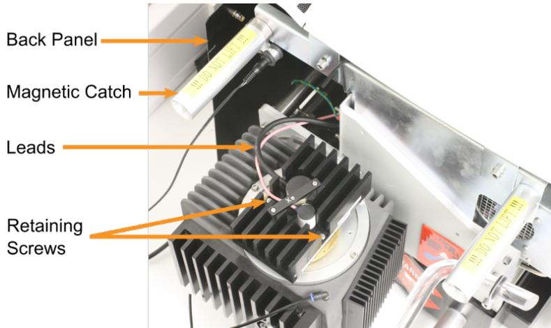
*Figure 114: Lamp housing fittings with lamp cover removed*
