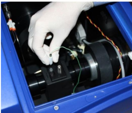
Figure 5: Inserting the in-sample temperature probe
