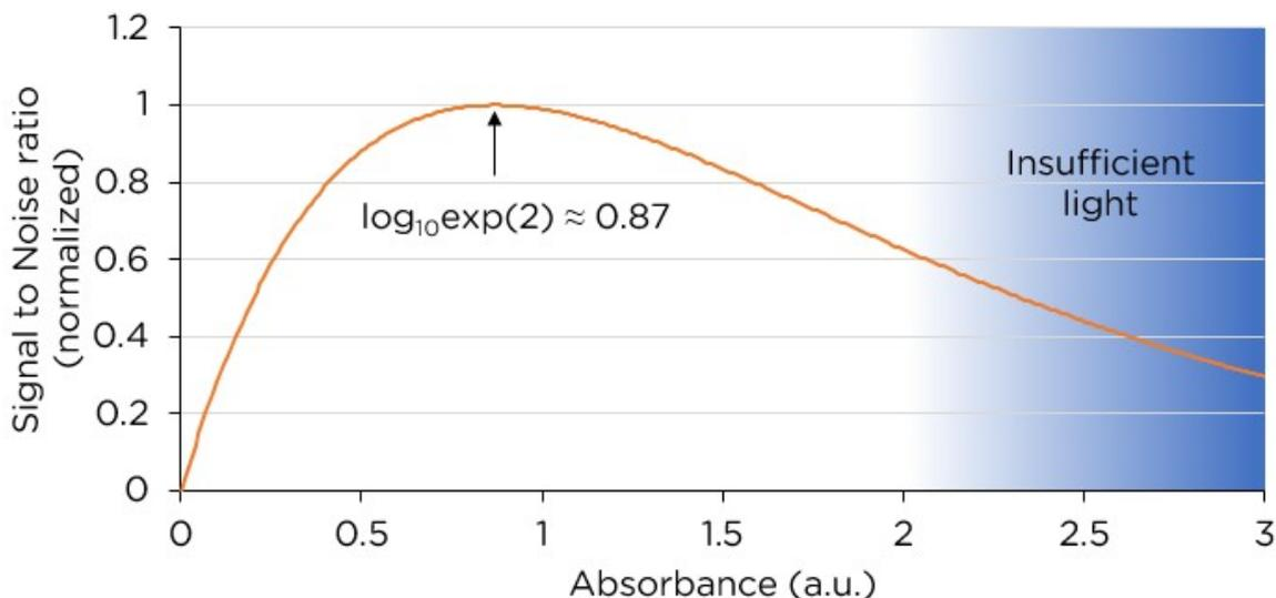
Figure 105: Signal-to-noise ratio as a function of absorbance.
