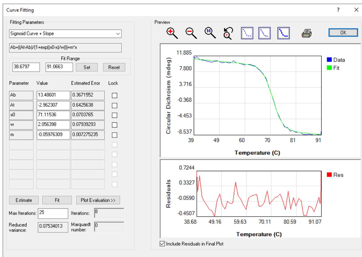
Figure 85: The Curve Fitting dialog
