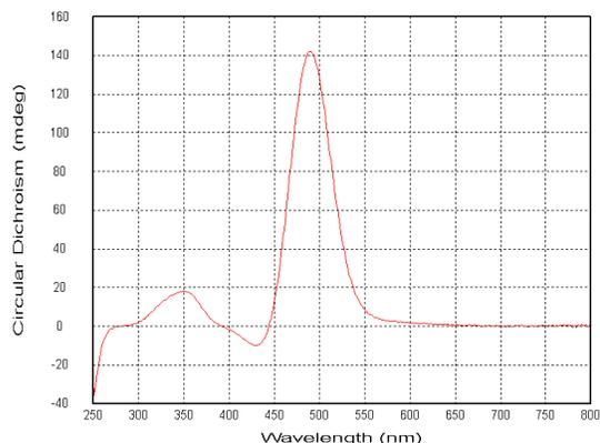
Figure 111: CD spectrum of tris(ethylenediamine) cobalt chloride
