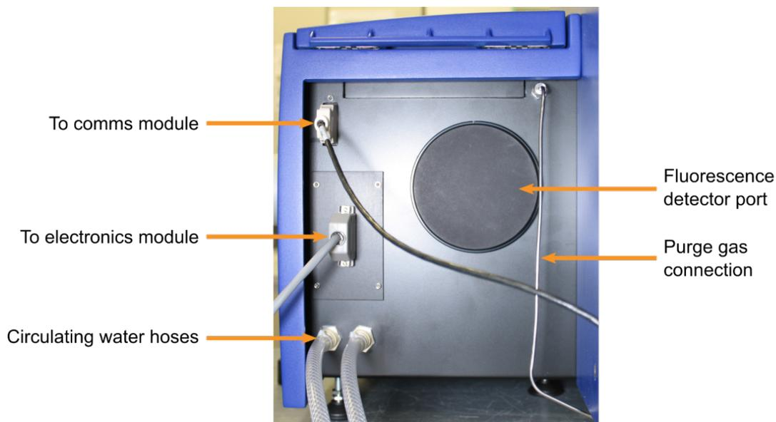
*Figure 14: The rear of the sample chamber*
