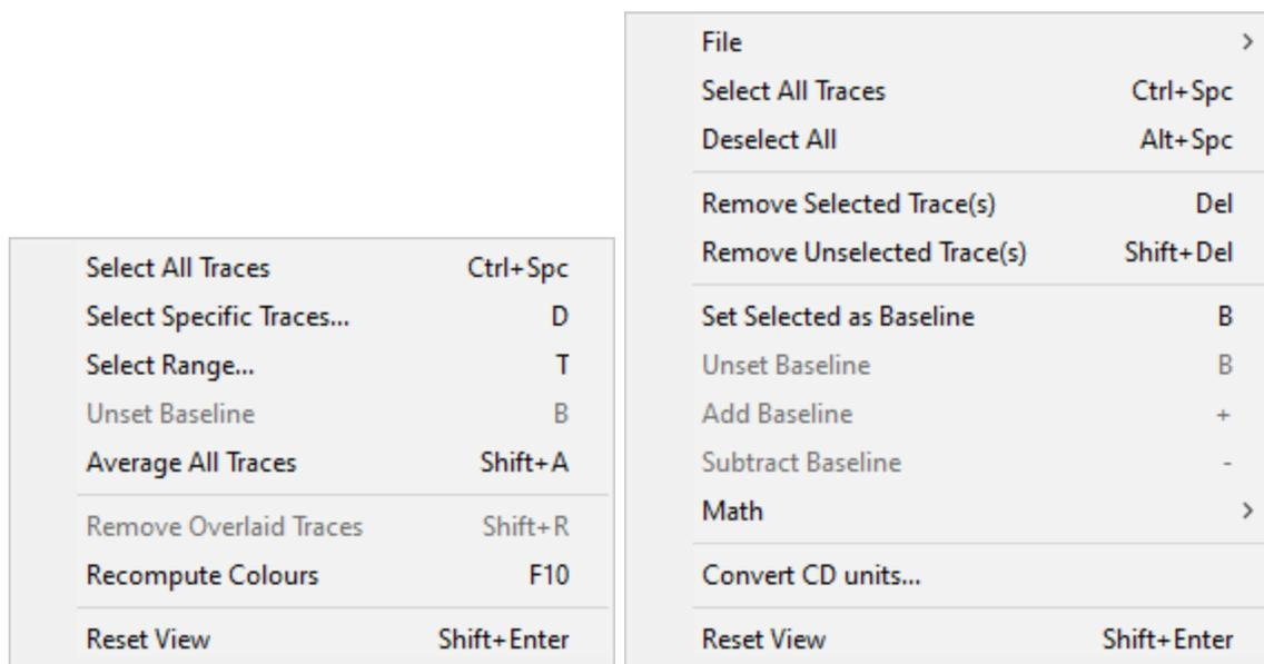
Figure 79: The Graphical Display right-click menu with no (left) and a single trace selected (right)
