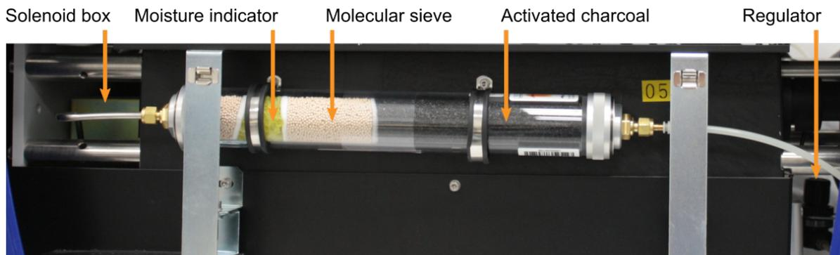
Figure 12: Components of the nitrogen purge gas flow
