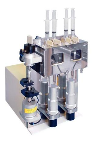
Figure 3.41: sequential-mixing SHU in sequential-mixing configuration
