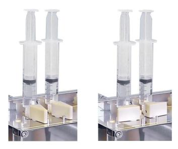
Figure 3.12: drive valves in Drive position (left) and Load position (right)
