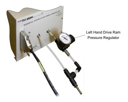
Figure 3.45: position of the drive pressure regulator on the rear of the SHU
