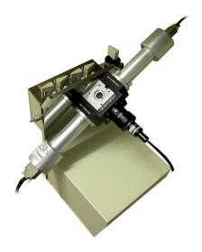
Figure 2.20: the fluorescence polarisation accessory
