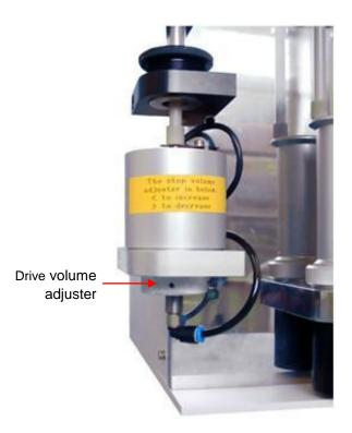
Figure 2.6: the location of the drive column adjuster on the stop mechanism
