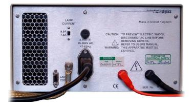
The Lamp Cont socket on the rear of the PSU not currently used.
