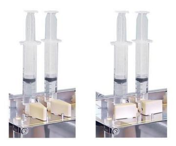
Figure 2.7: drive valve drive (left) and load (right) positions
