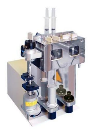
Figure 2.4: sequential-mixing SHU in single-mixing configuration
